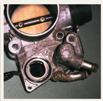
**Above:** To see a throttle body from this angle, you have to get it out of the car. The two hose nipples on the right are the coolant inlet and outlet for the fast idle control device. As you can see in this photo, the fast idle control device is attached to the bottom of the throttle body.
