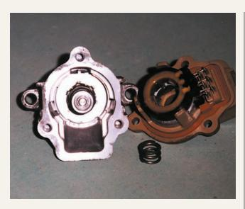
**Above:** Only three screws hold the cover on the ISC servo motor. Here's what one looks like opened up. The hefty-looking spring helps to seat the plunger.
