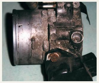
Above: The recessed idle air bypass screw is on the top of the throttle body. Make the idle speed adjustment here. In this photo, the black rubber plug that covers the screw is missing, which allowed moisture to collect and seize the screw. Putting the plug back when you are done will save a lot of grief down the road.
