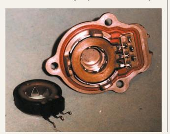
1157 bulb has two brightness levels with only three wires connected. The ECU grounds (pulse-width modulated, of course) the coil windings to move the plunger back and forth, opening and closing the idle air passage. If you think 'giant steps' and 'baby steps,' you'll better understand the reason for two opening coils and two closing coils.
