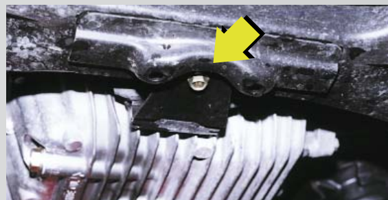
Figure 22: Don't jack up car by the control arms. In front, use this reinforcement (or the reinforced areas on the longitudinal rails, provided for the scissors jack).
