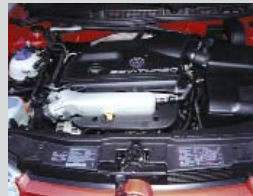
Figure 14: It's a Volkswagen Jetta GLS, and the engine label says VW, but catch the reference to a 20-valve turbo. The engine is taken from an Audi A4 and turned sideways, similar to the Audi TT, but with somewhat less power.
