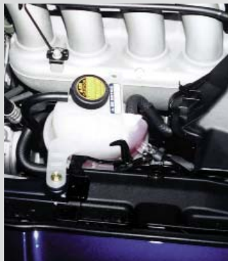
Figure 9: With the Celica beauty cover off, you can see the pressurized coolant reservoir. In this aerodynamic front-end model, the reservoir is not at the high point of the cooling system, so it has to be unbolted and raised (also freeing some hoses after loosening the air cleaner cover). The reservoir can rest on the hood latch.
