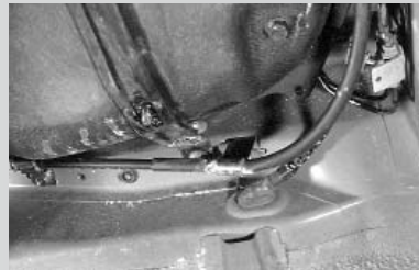
Figure 24: However, you must drain the main fuel tank before you try to get to either main or sub-pump. Remove drain plug shown.
