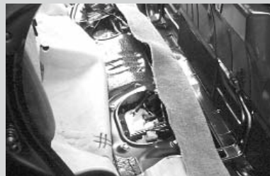
Figure 23: The saddlebag fuel tank is under the rear seat, and once the seat is out, you have access to the pump assemblies.
