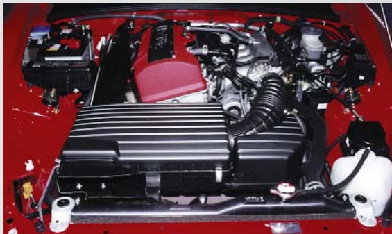
Figure 20: The engine compartment of Honda's sports car convertible, with its north-south, 2.0 liter four cylinder that develops 240 naturally aspirated horsepower. Notice the huge air cleaner. The engine revs over nine grand, and at that rpm it really inhales.
