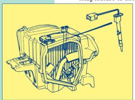
the evaporator from freezing up. It does this by cycling the compressor clutch ON and OFF as necessary. If the thermoprobe fails, it will most likely allow the compressor clutch to engage initially, then open the compressor clutch circuit. The compressor then remains OFF and the A/C system produces poor cooling.
