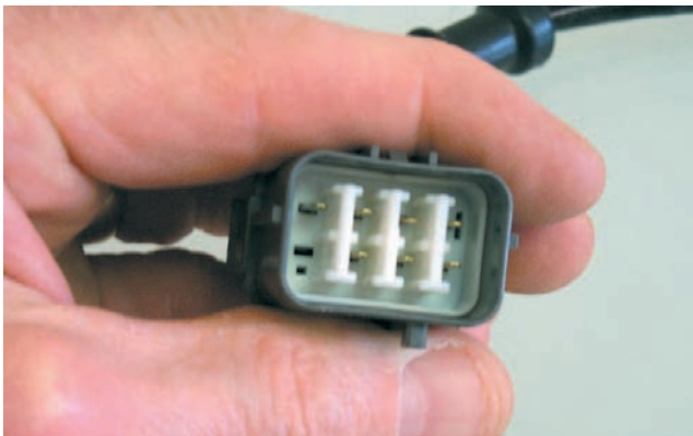
Linear Sensor Connector: The linear sensor has an eight-terminal connector, but only seven of them are occupied. Of those seven, only five are doing any work.
