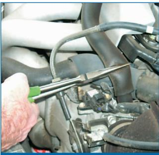
If the idling engine suddenly runs smoothly with the PCV line closed, you know something is wrong with the PCV system. Either the valve is locked open or the hose has gone porous upstream of your pinch.
