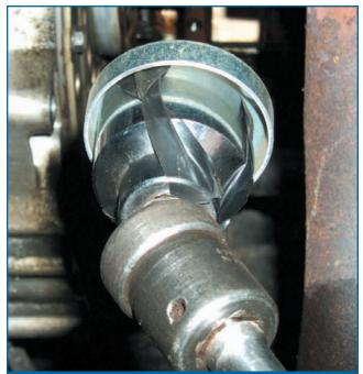
A third hand in a tight spot could do a lot. If you don't have one, though, sometimes a swatch of black tape can work to hold a freeze plug on the extension when you have to reach in where no human hand can fit.
