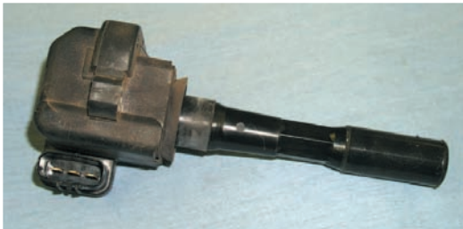
Above: Could hardly be simpler. Two terminals are the primary circuit; the third is the ground for the secondary (but read the text for why you can't check that last).
