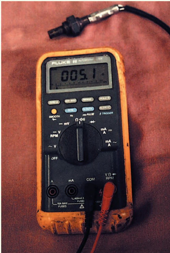
Figure 2: A simple digital multimeter (DMM) is all that's needed to test oxygen sensor heater resistance, but the test temperature is critical. Never check the resistance of a hot sensor heater and then just compare those readings to the manufacturer's specification. Manufacturers' specifications for heater resistance are given in connection with a specific temperature (usually room temperature). Heater supply voltage and ground can also be checked with the DMM.
