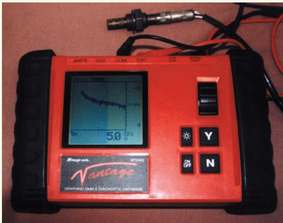
Figure 3: A graphing multimeter (GMM) can be used to test the oxygen sensor heater as well. A GMM provides a linear graph of the heater resistance as the temperature of the heating element changes. Current can be graphed with a GMM as well.
