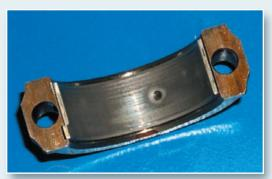
The bearings, main and rod, were worn, though not disastrously so. The engine uses a gang-saddle for all the main bearings, allowing you to flush out most of the oil galley in the parts cleaner. Nonetheless, there was enough wear to put in a new set of standard shells, checking them with plastigage.
