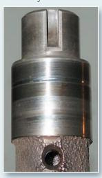
The camshaft lobes and bearings showed only minimal wear, but the seals had worn grooves in the front of each cam, just inboard of the timing sprockets. You could put new cams in, I guess, and maybe they make oversize seals and repair sleeves for these cams, but there is a bit of variability to just where you put the seals. So with a bit of care, you can put them so the lip rides in a new spot on each cam.
