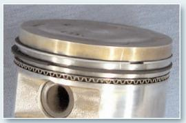
The pistons, coated with the usual surface of carbon and varnished in the ring area enough to lock some of the oil scrapers in place, cleaned up fairly well, and the new rings moved freely but not too freely in their just-excavated grooves.
