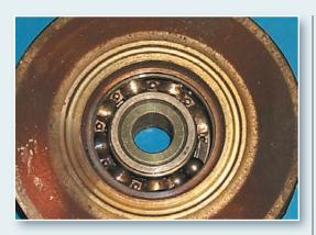
No doubt there would be this and that else, plugs and filters, accessory drive belts and such – the A/C idler bearing had disintegrated and locked the pulley, but most things were caught in plenty of time – no aluminum-fouled spark plugs or other exotic failures. The engine was still running normally on
