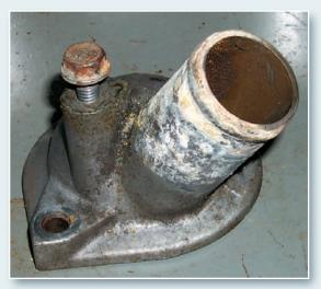
Obviously, the oil had distorted the rubber of the thermostat gasket, but there was the possibility that it seeped into the wax pellet as well, rendering the 'stat unreliable. Close by, an important problem-preventive on any Honda system comes with cleaning up the thermostat housing, in particular the small boss where so many different circuits find their ground return. If that ground grows resistance, you can find many hard problems resulting.
