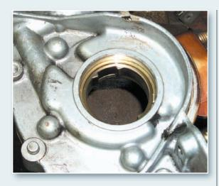
So, I held my breath and just re-used it uninspected, carefully replacing the crankshaft seal and packing the pump with lubriplate grease to prime the lubrication system at first crank.
