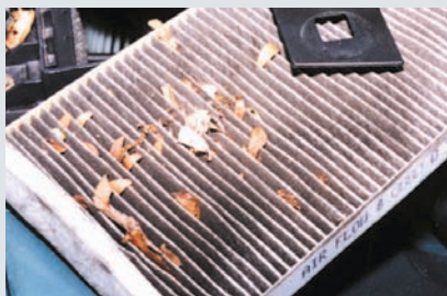
Figure 18: But when the plastic shield is removed and we pull out the filter, it shows a surprising amount of leaf debris after just a few thousand miles.
