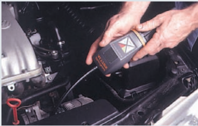
Figure 10: An R-12/R-134a-compatible conventional leak detector that meets the most recent leak detection standards is an acceptable substitute to find refrigerant leaks when trace dyes are not permitted by the manufacturer.
