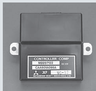
Figure 12: The belt lock controller is a separate electronic module as shown, or it may be part of the A/C module ("amplifier") on Japanese cars where the A/C compressor shares a drive belt with other accessories.
