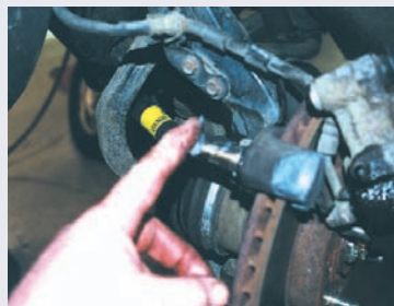
Photo 8: During a Honda brake job, the most commonly overlooked and most frequently underserved components are the caliper slides. Make sure the seals are not cracked or torn and lube up those slides. Dow Corning 111 works well
