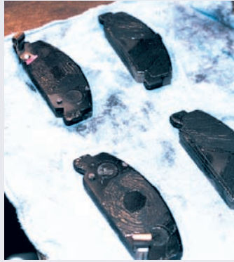
Photo 6: Factory pads come with a packet of moly. This goes on the pad ears, between the shims and against the caliper surfaces. Make sure the caliper spring steel guides are rust-free and the caliper surface behind the caliper guide is rust-free. When installing pads, they should slide right in place with no 'persuasion' necessary.
