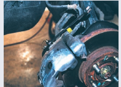
Photo 7: To avoid trashing an aging master cylinder, open the bleeders before squeezing the piston back into the caliper. If pressing back the piston requires any significant effort at all when using large pliers, the piston may be rusty and need replacement. Complete caliper replacement is another option if you're so inclined.
