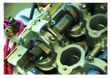
The eccentric bolt forces parts A and B away from one another. Because part A can't move (it's wedged against the cam lobes), the only thing that can move is part B. Part B moves by forcing the shim buckets downward, away from the camshaft.
