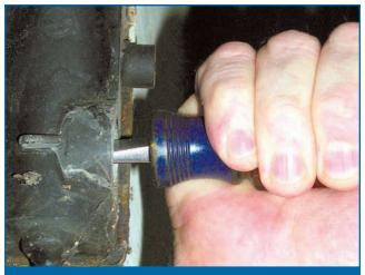
It's an unpleasant surprise when the plastic butterfly snaps off the radiator drain cock. To remove the broken piece from the radiator, heat the tip of a stubby screwdriver and stab right into the plastic stump.
