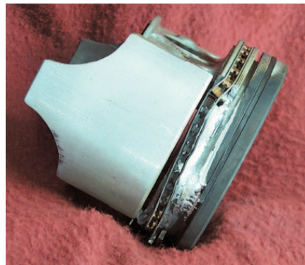
Detonation blew the rings through this piston's lands and grooves.
