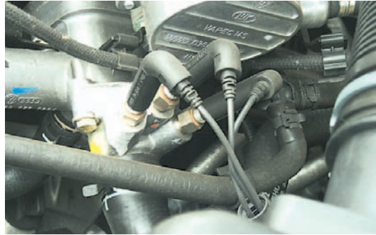
The VW TDI produces so little waste heat it includes three electric heaters for coolant headed for the heater core.
