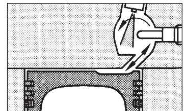
Combustion chamber shape and nozzle location for the swirl chamber system
