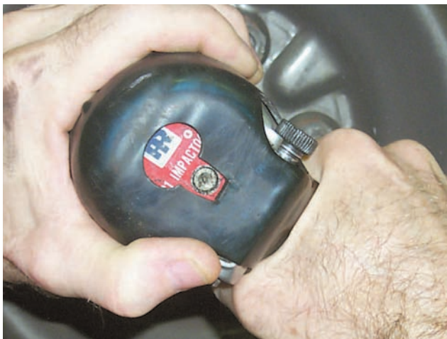
Airwrenches can put out tremendous torque. Enough to bend hubs and wheels or stretch wheelstuds and strip the threads out of nuts. That's not the way to tighten a critical fastener.
