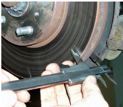
The cast-iron 'meat' left on a brake disc can determine whether it converts all the vehicle's motion to heat, or whether it just gets hotter and hotter.
