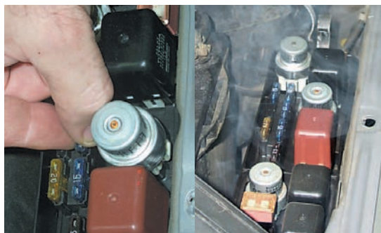
Replace that troublesome and often-blowing fifteen-amp fuse with a larger current version, and you could let the smoke out of the wires.
