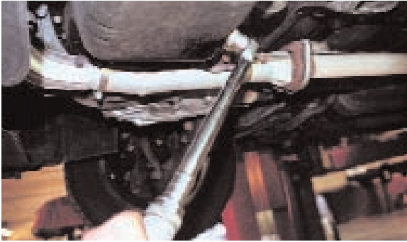
Photo 1: I can't overstate the importance of replacing the oil drain bolt aluminum washer every time you change oil, and torquing the bolt to 31-33 lb.ft. If you try to tighten the old washer, you'll stress the bolt and the pan until the threads are junk, the pan's distorted and can't seal.
