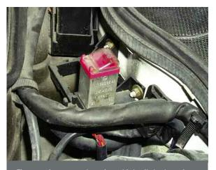
The overvoltage protection relay, with its distinctive red cap and fuse, takes the hit if there's a voltage spike. But it shuts off the fuel or the spark or both when it does so. This should be your first check if a car has gone dead unexpectedly. Be sure to locate and repair the cause of the overvoltage before you finish the job.
