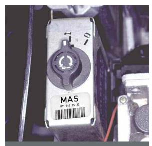
In later vehicle systems, the work of the Klima relay is part of the various tasks of the MAS control unit. Besides its responsibility for fuel and ignition circuits, it also cycles the air conditioning compressor or, as does the Klima relay, shuts it off entirely if the shaft speeds do not correspond.
