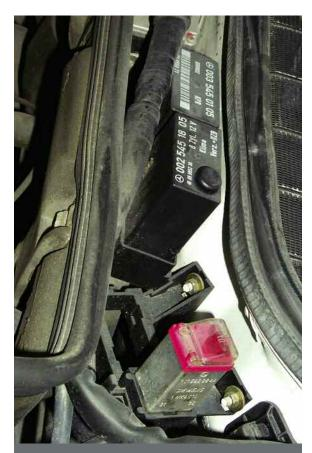
If the air conditioning compressor won't engage beyond the first couple of turns when it first tries to connect, the problem may not be electrical at all. You may just have a loose drive belt, apparent to the Klima relay as a lack of correspondence between the compressor speed sensor signal and the crankshaft speed sensor. It disconnects the compressor to save the belt.
