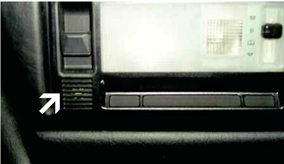
At the lower left corner of the courtesy/dome light is a small grille behind which is the cabin temperature sensor. A tube from it leads behind the passenger side outlet duct, where a small air pump constantly draws fresh air through the tube and over the sensor.
