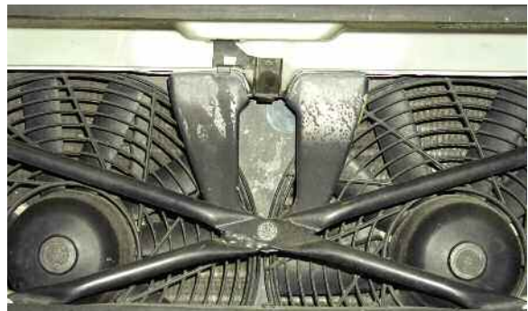
Mercedes-Benz usually includes a pair of auxiliary fans for cooling the air conditioning condenser in front of the radiator. Relays control these fans and their speeds, in response to command signals from the control unit. These pusher fans mean the air conditioning system can work effectively even at low speeds in very hot weather.
