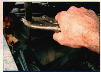
A broomstick or shovel jammed under the hood can stab the radiator or other parts and can fall out if you bump it. If the car you're working on has lift cylinders to hold up the hood, but they've lost their lift, lock them in place with your trusty Vise-Grips.
