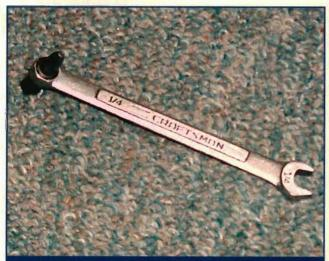
It's a rare offset screwdriver that can deliver much torque to an inaccessible screw, but glue a #2 Philips bit into a quarterinch box wrench, and you can get almost anything to move. Grind the blunt stub of the bit off if you need to for even more clearance.
