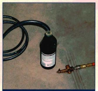
Sometimes it's very hard to get 90-wt oil to flow uphill through a line into a transmission or differential. One way to try – with some care! – is to route the oil through a fuel line with one end in the casting and the other over the greasebottle tip. Then hold the bottle upside-down, poke a small hole in it and judiciously introduce air pressure into the bottle to push the grease through.
