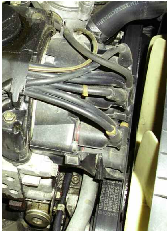
Spark must travel through the same sorts of circuits on a Mercedes-Benz as on any other vehicle. Check the wires for continuity, inspect the cap and rotor for carbon tracks, cracks and even carbon-button failure.
