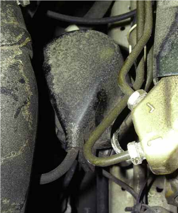
This cover protects the ignition coil from the elements, but also can form a path for a carbon track. When you check the coil for continuity and physical damage, make sure to inspect the coil cover as well.
