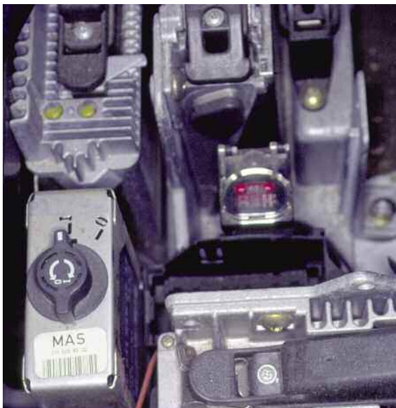
Mercedes-Benz vehicles have a formidable array of control units, not just in the front compartment shown here but in many other places in the vehicle. Many control units, however, does not mean the problem is in a control unit. Before pursuing the most complex possible diagnosis, check the fundamentals – fuel, spark, compression and timing – for proper operation.
