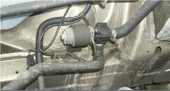
Two electrical components play important and interconnected roles for heat and defrost. The auxiliary water pump, top, circulates coolant through the heater core as needed regardless of the circulation through the engine's main water pump. The monovalve, bottom, opens or closes the coolant's hydraulic circuit to and from the heater core.
