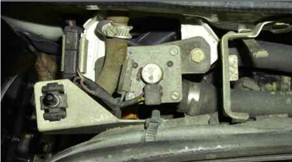
Two electrical components play important and interconnected roles for heat and defrost. The auxiliary water pump, top, circulates coolant through the heater core as needed regardless of the circulation through the engine's main water pump. The monovalve, bottom, opens or closes the coolant's hydraulic circuit to and from the heater core.
