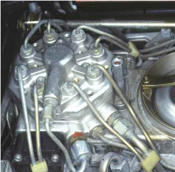
For many years, all the way up to this 1992 model, Mercedes-Benz used increasingly complex versions of the Bosch CIS-E fuel injection system, with continuous injection and a fuel distributor as here.
