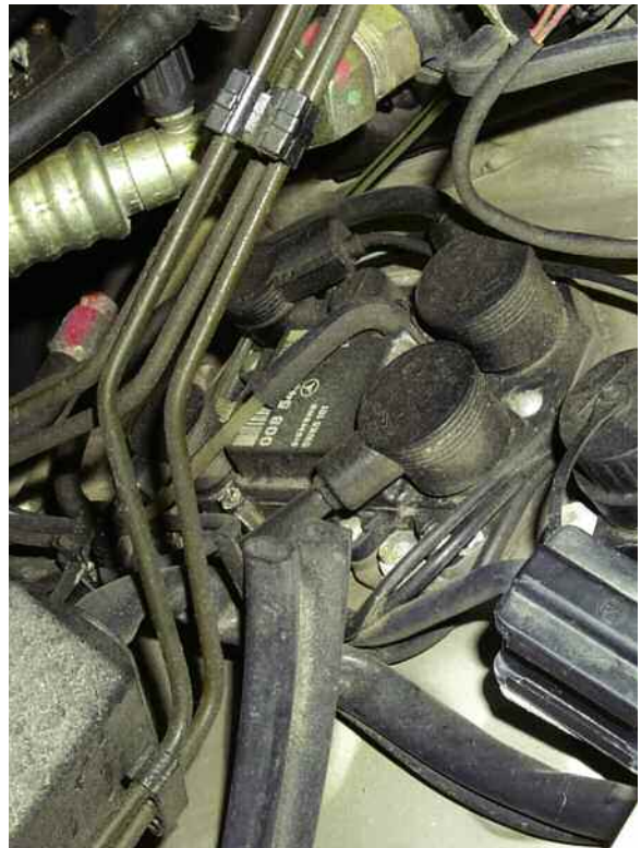
The ignition module is responsible for triggering the coil, that is, interrupting the ground circuit so the electromagnetic field collapses and generates the high-voltage secondary spark. Check your service information to see just what information in the form of voltages you should find on the module's terminals, because this varies by model and by year.
