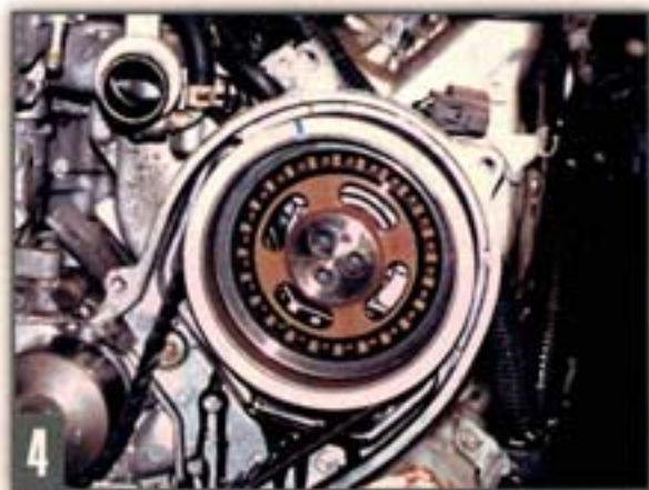
Always take the bolts out of the cam sprocket before removing the timing belt when replacing the water pump. You need the belt on to keep the pulley from turning, even when using an impact wrench to remove the bolts. The black slime from the sensors is normal, so don't sweat it, but the green crust below the lower left water pump bolt isn't. There's not much sense sending an engine out the door unless it's capable of going another 90,000 miles. Convince the owner to replace the water pump and timing belt.
