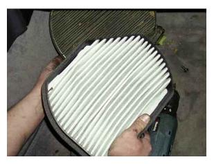
Current Mercedes-Benz models use cabin filters, sometimes two in series, to clean the incoming air to the passenger compartment. When there are two cabin filters, the first is an electrostatic particulate filter to catch dust and pollen, and the second is an activated charcoal filter to remove vapors. Each vehicle owner's manual lists the corresponding replacement interval, though under particularly dusty (or malodorous) conditions it may be advisable to replace them after a shorter interval.
