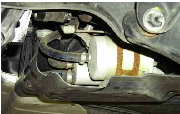
Pump and filter
