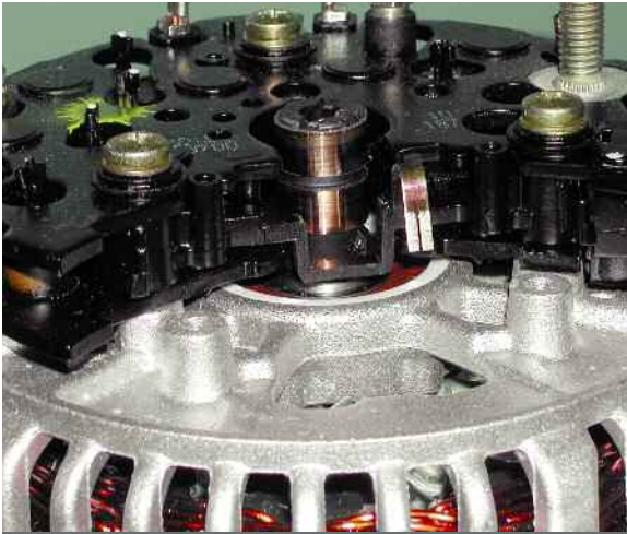
With the regulator and brushes removed, the slip rings are visible surrounded by the rectifier. The tab to the right provides output voltage to the regulator
