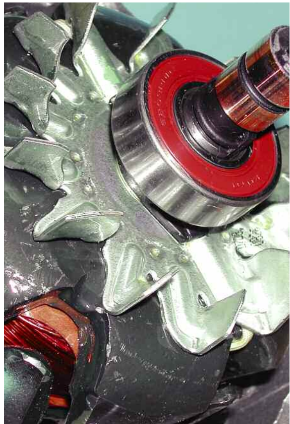
Inside the alternator is the rotating armature, supported at either end by bearings, with a field coil powered through the slip rings and ferrous metal 'fingers' that focus the magnetic field produced by the field coil. The centrifugal fan draws cooling air through the alternator.
