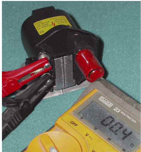
A conventional ignition coil, the type found on most Mercedes-Benz vehicles, uses primary and secondary circuits that share a connection at the battery-positive terminal. The primary circuit tested here builds an electromagnetic field around the iron core of the coil. Resistance through this and all other primary circuits is relatively low.
