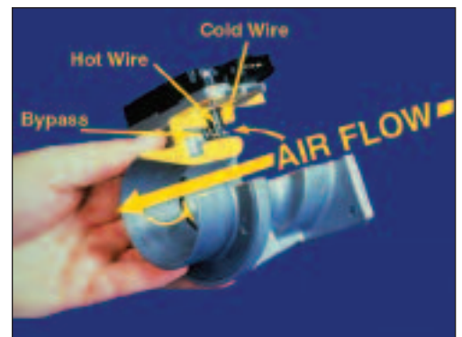
Air Flow Meter
