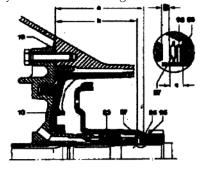
In the absence of shavings, remove the transmission, remove the front cover and replace the thrust washer and compensating shim. Measure the axial play of clutch K1 and correct if needed (see job 27-640, step 83). Flush the torque converter and coolant lines clean. If you find steel shavings in the cleaning fluid (usually kerosene), replace the torque converter.
