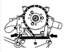
If oil leaks where the five parts meet between the cylinder heads gasket and the cover gasket, remove the top front cover and its gasket. Apply one drop of Loctite 5900 sealant to the right and left ends once they're entirely oil-free. This fills the gap between the cylinder head gasket and the cover gasket. This repair can't work if the parts are not entirely free of oil!
