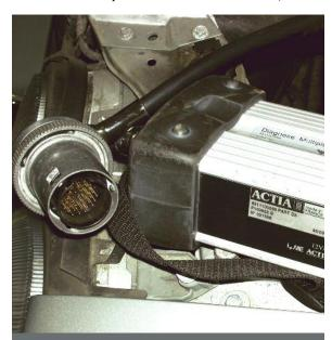
The terminal is common to all Mercedes-Benz vehicles within the production range. The box serves to sort out the information, to protect the diagnostic computer and to identify the specific car. This box is the interface between the car's computer and the diagnostic computer
