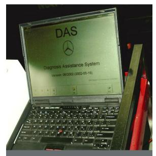
The Diagnostic Assistance System is the current Mercedes-Benz factory diagnostic software system. If you do enough work on Mercedes-Benz cars, it is probably worth your while to invest in this equipment. It allows full access to each computer-controlled system on the car. While it can't tell you the tire pressure yet, don't count on that being permanently out of the system's reach.
