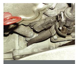
Cam sensors have become more important as engine control systems have become more complex. Originally they served principally to sequence the fuel injection systems once Mercedes-Benz went from the CIS-E systems to the SFI systems. But as camshafts become themselves variable, the performance of the engine, both in terms of emissions and in terms of output, the sensors had to become more and more sensitive.
