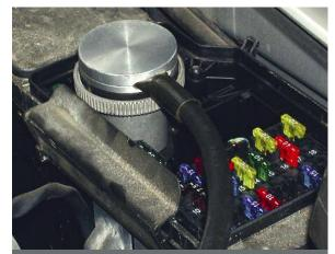
The diagnostic tool connector is the gateway to the interface for whole system diagnosis. It fits precisely into the diagnostic socket and locks in place with its thread. Coupled with the rest of the diagnostic equipment, this can allow access to current operating parameters and those recorded in the various histories of the on-board systems. Connected through the proper interface devices to a laptop, it can record and display information either in the workbay or underway on the road.
