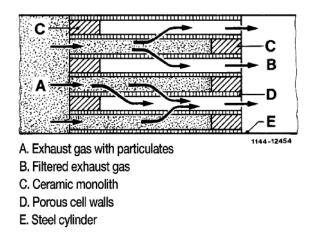
Present Diesel exhaust traps consist in a fine ceramic filter to catch particles of soot. When enough of them collect, they burn off in the exhaust. Later versions of Diesel exhaust treatment use reducing catalysts to remove NOx from the exhaust.
