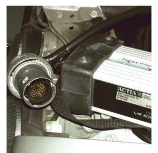
The terminal is common to all Mercedes-Benz vehicles within the production range. The box serves to sort out the information, to protect the diagnostic computer and to identify the specific car. This box is the interface between the car's computer and the diagnostic computer
