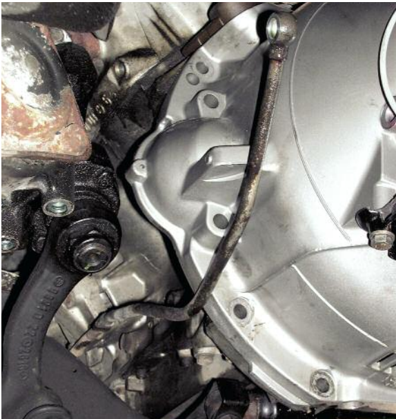
Next, unbolt the right and left side bellhousing bolts, with the transmission jack securely supporting the weight under the transmission pan.
