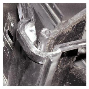
The likelihood of finding a replacement door for a 20-year old car never built in huge numbers didn't seem high, at least in the short time available before the owner expected the vehicle back. But there are so many work-hours involved in the job, the prospect of gluing the stub of the pin on and hoping it would hold was disconcerting.
