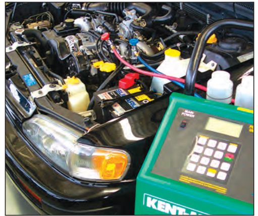
Recovering Refrigerant and Oil
