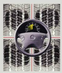
Straight ahead, accelerating. We i m m e d i a t e l y notice the weightshift to the rear tires, evidenced from the increase in the relative size of the rear treadpatches. Since the total weight of the car doesn't change, however, the total area of
