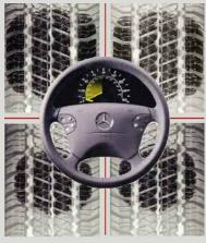
Straight ahead, braking. Again we see the weight-shift from a speed change. The front treadpatches have now grown larger than they were in steady cruise. We can also see the suspension of this car is sufficiently sophisti-
