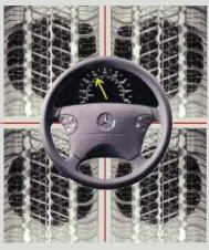
Straight ahead, s t e a d y s p e e d . Assuming the inflation pressures are identical for all four tires, we see there is slightly more weight on the front tires than on the rears, typical for front-engined
