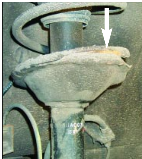
Inspecting Spring Near Seat (arrow)
