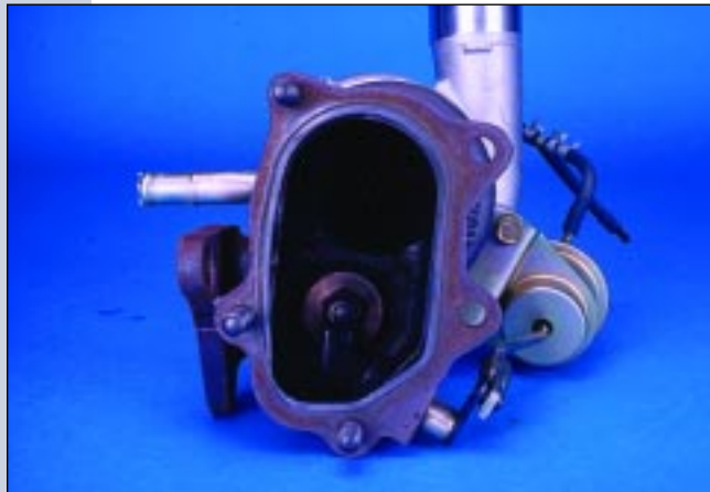
Wastegate Valve Inside Turbo Housing
