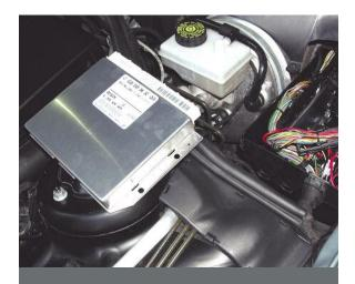
The information from all the sensors we've described in detail, as well as data from the engine and transmission controls, flows into the ESP control unit, here unplugged and visible from the side. All the read-only memory for allowable thresholds, all the calculations to determine what the car's situation is and what steps, if any, to take for correction, as well as the output signals to the traction control actuators, center here.
