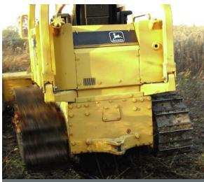
It's the simplest of all steering systems: Stop one side, and the 'dozer grinds in a circle around it.
