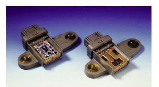
Mounted as close as is practical to the very center of the car, the lateral acceleration sensor detects lateral acceleration and sends quantified information about that in the form of a millivolt signal to the control unit. The sensor itself is Hall-effect, but the internal microprocessor translates the data into a scalable signal.
