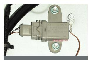
The lateral acceleration sensor is relatively delicate, about like the bulb in an incandescent troublelight, though it can sustain the bumps and shocks of the moving car. If you remove it for test or replace one, however, be careful not to drop it on the floor or smack it against a workbench or hard parts of the car. The exclamatory red label on it reports (in German) that it's sensitive to impact damage.
