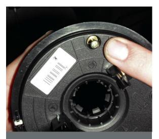
The steering wheel position sensor can only fit over the splines and onto the column in one position, but the internal 'clock' spring could be wound beyond the correct position with the sensor on the bench. Then the spring could snap when the steering wheel turns to the tight extreme. To prevent this accidentally happening, leave one of the attachment screws in the sensor to keep the rotating part lined up with the stationary plate.
