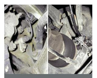
All of the intertwined traction controls, from ABS, through ASR to ESP, depend critically on the wheelspeed-pulse information from each wheel. These induction sensors provide the fundamental data on vehicle speed and on variations at each wheel. If a single one of them stops working, the whole interconnected set of traction-control systems turns off; the car drives as a normal car without traction control; the warning lights turn on as a DTC takes up residence in memory.
