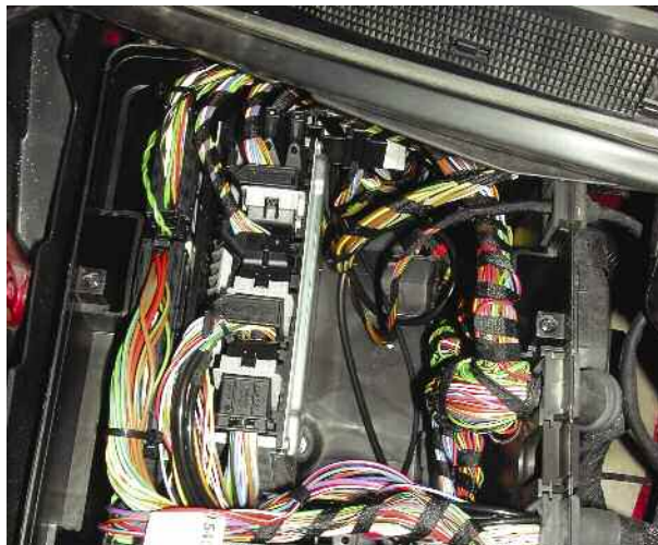
Circuits, hydraulic and electrical, are the muscles and nerves of the ESP traction controls. The hydraulic control unit straddles the brake lines between the master cylinder and the four calipers. It includes the pressure pump and the solenoid valves for all ABS, ASR and ESP actuations. The control unit resides in the electrical control unit compartment, just in front of the bulkhead in most car models.
