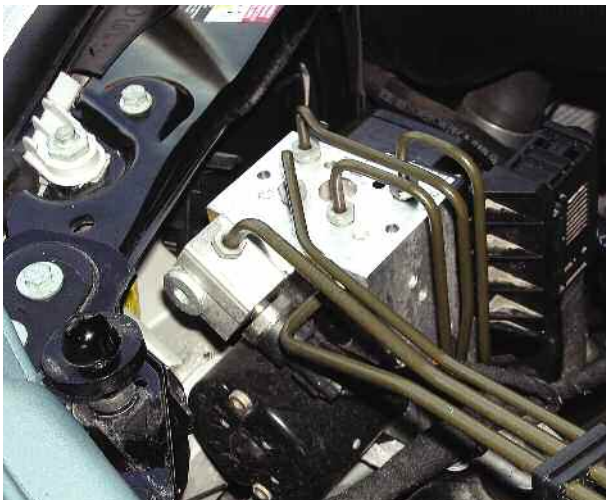
Circuits, hydraulic and electrical, are the muscles and nerves of the ESP traction controls. The hydraulic control unit straddles the brake lines between the master cylinder and the four calipers. It includes the pressure pump and the solenoid valves for all ABS, ASR and ESP actuations. The control unit resides in the electrical control unit compartment, just in front of the bulkhead in most car models.
