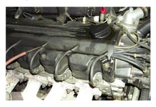
Worn spark plug wires don't necessarily look worn – they aren't the moving parts. Inside, the electrons can eventually start finding new paths to ground or burning the cables internally open enough to drive up the coil output to a threshold sufficient for idle, but not for any other engine load.
