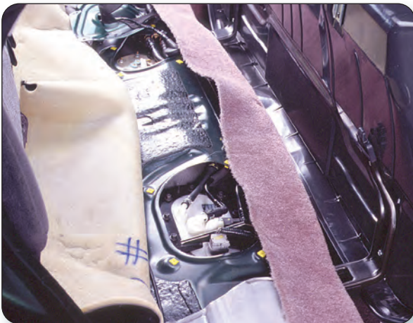
Figure 2: Fuel Pump and Sub Pump Unit Access
