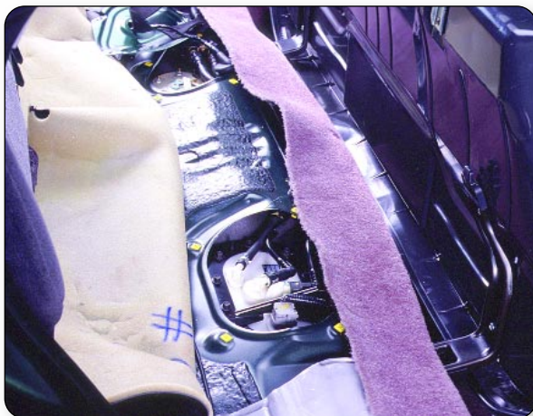
Figure 2: Fuel Pump and Sub Pump Unit Access
