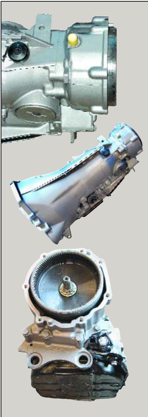
The transmission for 4MATIC is identical to the transmission for the car without that option, however the 4MATIC version includes a ring gear and flange on the output shaft of the gearbox.
