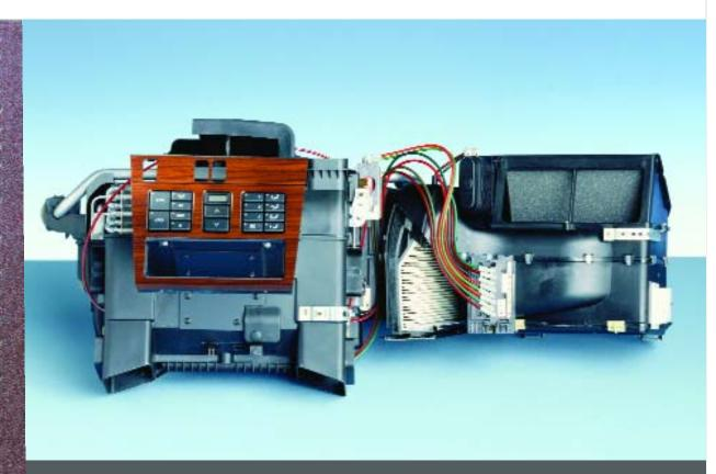
Slightly smaller and slightly simpler than some Mercedes-Benz systems, the 202 climate control nonetheless includes everything to do the job. The control unit behind the pushbutton plate, the boxes for the heater core and A/C evaporator, the ductwork, vacuum motors and lines to work the blend doors and finally, a dust filter.
