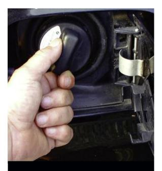
DTC P0442 or P0455 may be set most often because somebody didn't install the gas cap properly, but don't automatically jump to that conclusion because real system leaks are also a possibility.
