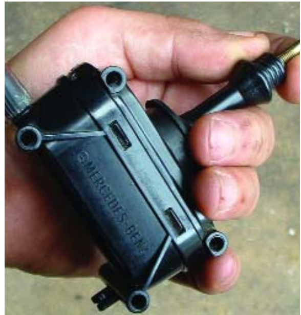
The operating elements are all pretty much the same. You screw the rod in or out to achieve the proper length.
