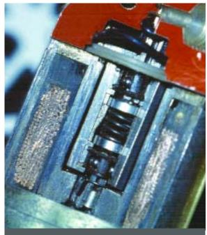
The sophisticated electronics of ABS won't be able to do their job if the tiny hydraulic passages and the electrohydraulic components are gummed up.
