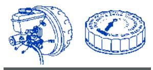
The master cylinder comes first in every brake bleed – not necessarily to bleed it unless you've replaced it or opened the adjacent hydraulic lines, but to draw most of the old fluid out by vacuum and replace it with fresh. On many Mercedes-Benz brake systems, check the reservoir cap to confirm the vent is open.
