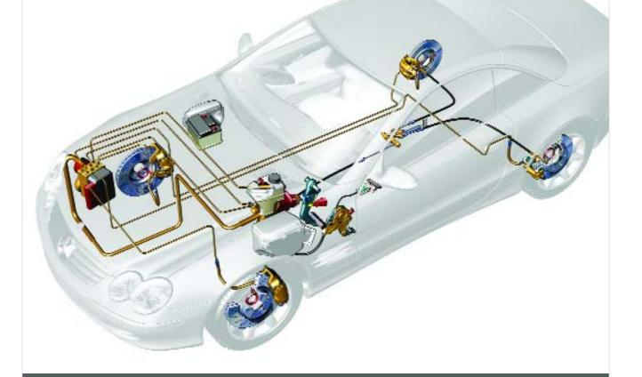
All hydraulic braking systems, from the oldest and simplest to the latest and most complex like this Sensotronic brake system from Mercedes-Benz shown in conceptual X-ray here, require the complete removal of all the air in the system to maintain hydraulic application force. They also all require periodic replacement of the fluid with new, both to remove any small debris that may accumulate and because the fluid itself changes boiling temperature over time.
