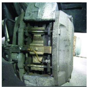
Bleed the front calipers next, keeping in mind that some late-model cars have more than one bleeder on the front calipers. While you're at work, carefully inspect pads, hardware and nearby suspension components. Don't wait for something to break.
