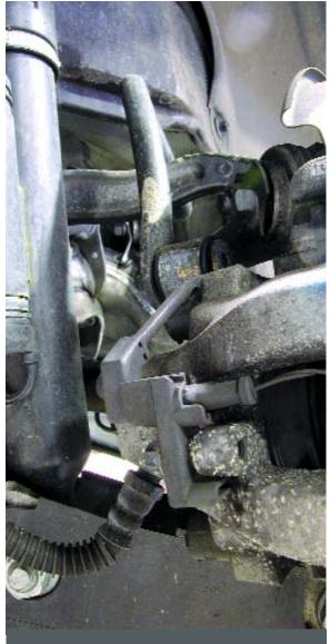
The bleed sequence proper starts as far from the master cylinder as possible, at the right rear caliper on most cars. Once you have clear fluid flowing from this bleeder, with no bubbles, you have a solid hydraulic path all the way back to the master cylinder reservoir. Then, move to the left rear.
