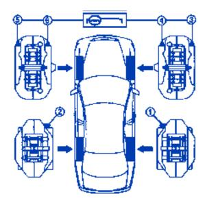
Every vehicle has a proper bleeding sequence to insure removal of all entrained air in the system. For virtually every Mercedes-Benz, start at the bleeder farthest from the master cylinder and work back closer one bleeder at a time. Make sure each circuit is flushed and without any bubbles before moving on to the next.
