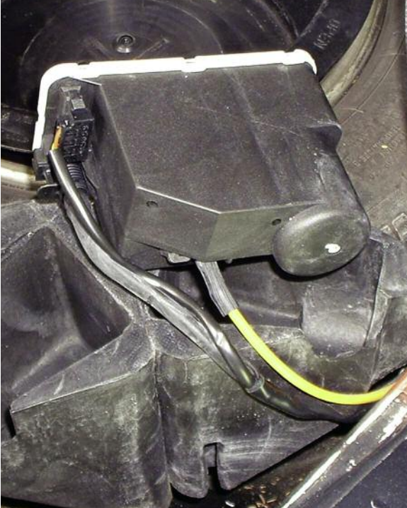
The pump may be found in the spare tire well, as in this specimen, under the back seat, or in the engine compartment. Note the single yellow vacuum/pressure line and the insulating foam casing.
