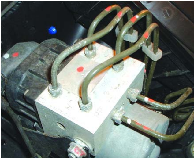
Tucked in unobtrusively under the hood, the hydraulic control unit translates electronic commands into action.
