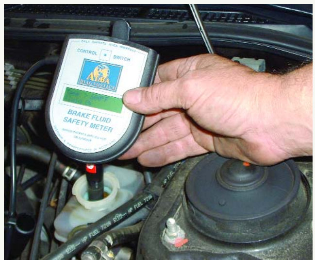
This tester hooks up to the car's battery and actually boils a sample of brake fluid to determine its moisture content.
