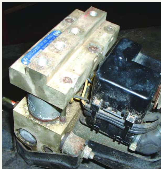
The common ABS-2S has its outlets in line on top.
