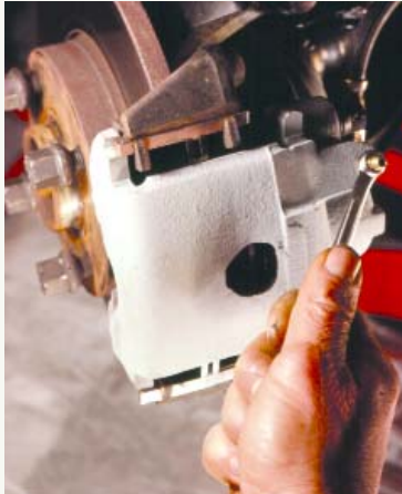
No matter how old the system, always open the bleeder before forcing the piston back.
