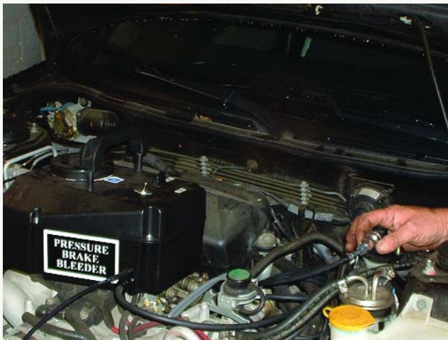
A flushing machine, such as this 12V unit, and a good set of master cylinder adapters make the job thorough, fast and profitable.
