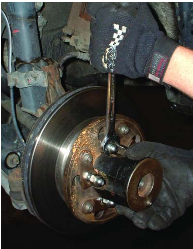
This is the universal adapter, but there are also those dedicated to particular bolt patterns.
